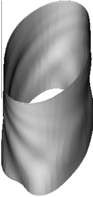
Fig. 8. The helical structure of 3D instability from the target experiment T1, visualized by the isosurface of vertical vorticity equal to 1.
